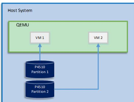
Figure 1: Example of 2 VMs in TLC Configuration
