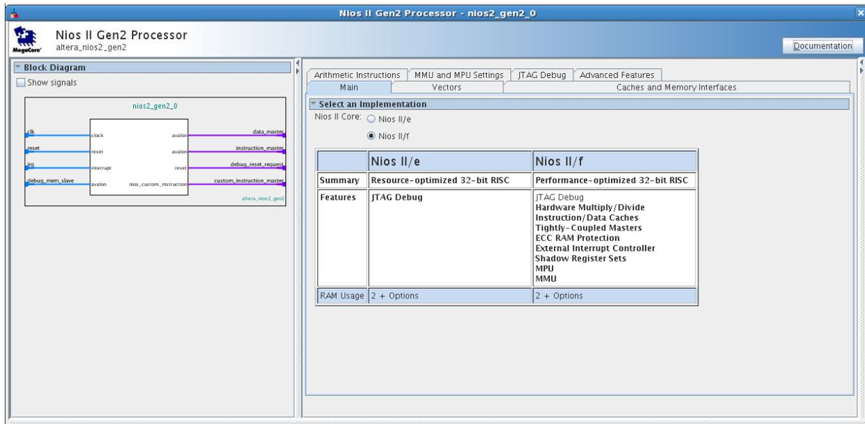
In Qsys instantiate a Nios II Gen2 processor and open the processor configuration window. Select the following settings in the tabs:
