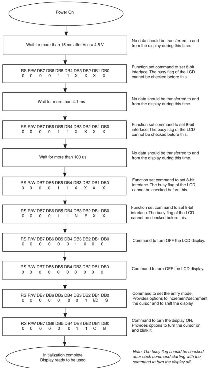
To simplify initialization, a delay of 15 ms is provided after each command is sent (instead of checking the status of the busy flag). However, while writing data into the LCD module, the status of the busy flag is checked after each data write. This makes the writing procedure faster.
