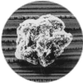
A dust speck landing on the chip's surface during fabrication ruins the chip.
