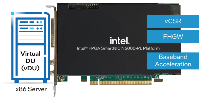
Figure 3. Using an FPGA SmartNIC accelerator to virtualize the CSR function
